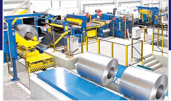
Cut to Length Line
